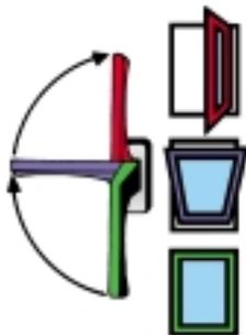
Position for cleaning or for a short period of ventilation. Do not leave the window unattended.
