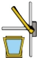
If the window opens or closes on its own due to air pressure or suction special fittings are available to overcome this. These must be fitted by a qualified person.
